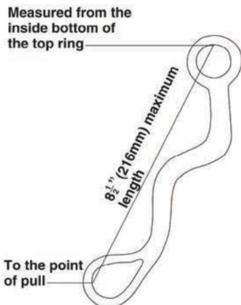
**Figure #2 - Bit Measurements**
